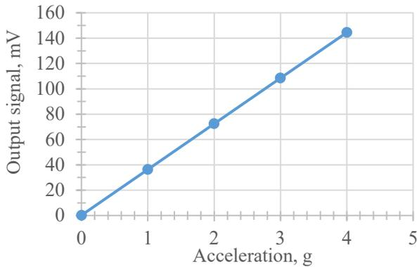
**Figure 5. Proposed sensor sensitivity (modelling results).**
