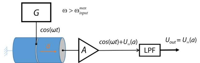
Figure 1. Design concept of a proposed microaccelerometer.
