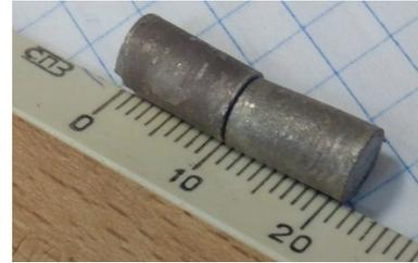
**Figure 3. Sensing elements made of CTS-19 that were simulated.**
