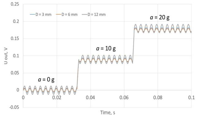
**Figure 8. Output signals from sensing elements of different diameter  $D$  (modelling results).**
