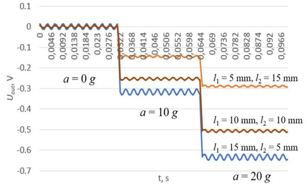
**Figure 7. Output signals from sensing elements with different ratio of sensing part ( $l_1$ ) and exciting part ( $l_2$ ) (modelling results).**
