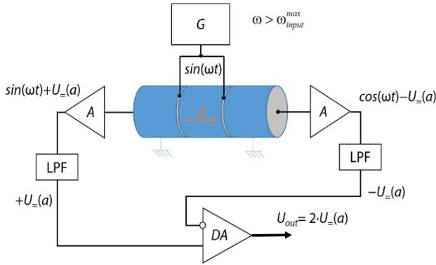
**Figure 2. Differential piezoelectric accelerometer design concept. DA: differential amplifier.**
