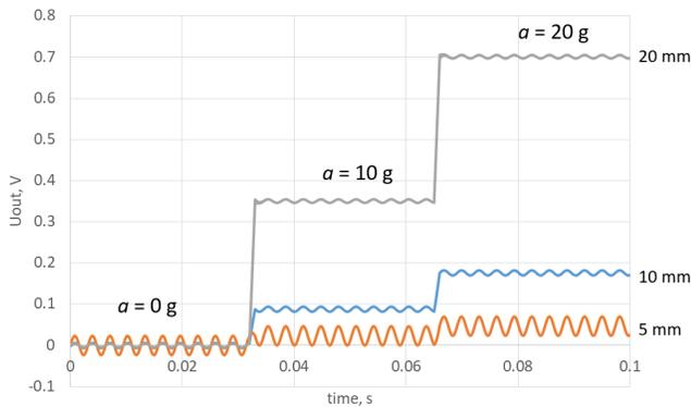
**Figure 6. Output signals from sensing elements of different length (modelling results).**
