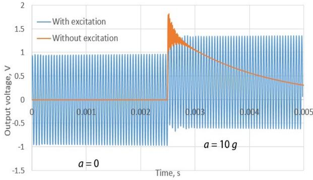
**Figure 4. Output signal at different values of acceleration (simulation results).**
